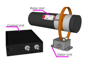
he telemetry system AXON J2T is designed for transmitting thermocouple based measurement signals from rotating shafts or other mechanical parts. Two sensors can be transmitted simultaneously. Like all AXON telemetry systems, the J2T is extremely robust and delivers reliable readings at operating temperatures of up to +140°C in continuous operation, even under the toughest conditions. The inductive, contact-free power supply of the Rotor Unit ensures an interruption-free operation.
