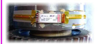
The highly effective inductive power supply of the rotating components allows an uninterrupted use even under harsh conditions.
