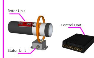
he telemetry system AXON J8T is designed for transmitting thermocouple based measurement signals from rotating shafts or other mechanical parts. Eight sensors can be transmitted simultaneously. It combines smallest possible design with extreme robustness and delivers reliable readings at operating temperatures of up to 140°C in continuous operation, even under the toughest conditions. The inductive, contact-free power supply of Rotor Unit and transducer ensures an interruptionfree operation.
